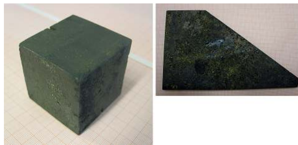
Figure 2. Photographs of the analyzed samples. Left: Heisenberg cube I (5 cm \times 5 cm \times 5 cm). Right: Wirtz plate (trapezoid with 18 cm base, 1 cm thickness; broken corner on the lower right).
