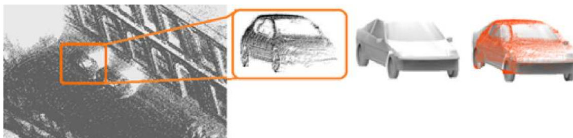
Fig. 7 Example of a 3D car model fitted and rendered to a point cloud
