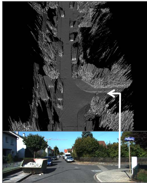
Fig. 4: Volumetric surface reconstruction. Top figure shows the 3D surface reconstruction over 250 frames (KITTI sequence 15, frames 1-250) with street image shown at the bottom. The arrow highlights the relief of the sidewalk which is correctly captured in the 3D model.
