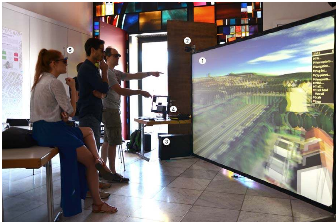
Figure 7. The mobile VR setup during a participatory process including a back-projection wall [1], tracking system [2], computer [3,4], a 3D-projector, and active shutter glasses [5] for the participants (photo credited to Dembski, 2019).
