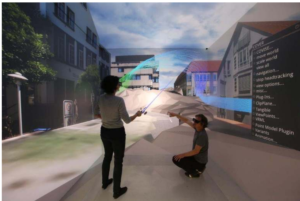
Figure 6. Particulate matter and wind flow simulation visualized in the CAVE. The particulate matter concentration is represented as an iso-surface. For the wind flow simulation, the color range from blue to green indicates wind speed from low to intermediate. The CAVE is a stationary five-sided cube for VR back-projection run by a 22-node cluster, five 3D-projectors, a tracking system, and active shutter glasses for the participants (photo credited to Wössner, 2017).
