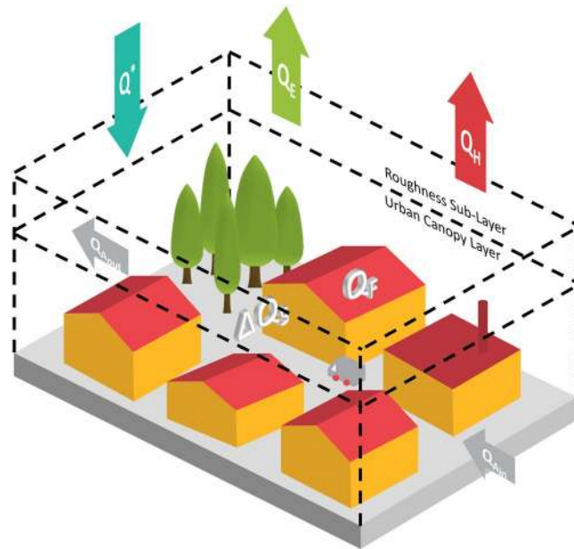
Figure 1. Conceptual illustration of the fluxes in the energy balance of an urban building–vegetation–soil–air volume. The equivalent surface energy budget per unit surface area through the top of the volume is: Q^* + Q_F = Q_H + Q_E + \Delta Q_S + \Delta Q_A ( \text{W m}^{-2} ), where, Q^* is the net all-wave radiation flux; Q_F is the anthropogenic heat flux (resulting from vehicular emissions, heating and cooling of buildings, industrial processes and metabolic heat release by people and animals); Q_H is the turbulent sensible heat flux; Q_E is the turbulent latent heat flux; \Delta Q_S is the net change in heat storage within the volume; and \Delta Q_A is the net advected flux. Arrows are drawn in the direction to which the corresponding flux is considered positive. \Delta Q_S and \Delta Q_A ( =Q_{A,in} - Q_{A,out} ) are positive if the internal energy of the volume increases.
