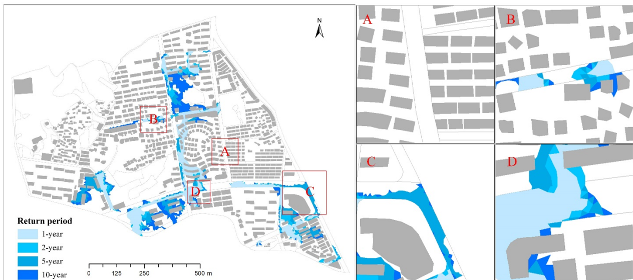
Figure 10. Inundation of the study area during different return periods ( t = 120 min and r = 0.4 ): (A) XJSR, (B) NLS, (C) AFR, (D) WSS.
