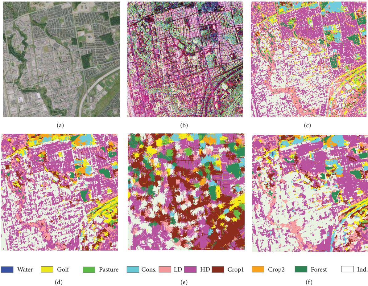
FIGURE 6: Zooming comparison of (a) Google Earth image and (b) PolSAR Pauli image and the classification results using (c) SVM, (d) NN, (e) SEM, and (f) DBN in an Ind. area.
