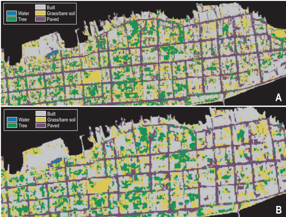
Figure 4. Masked sections of land use/cover maps of downtown Puntarenas City (see Figure 1) obtained respectively with (A) backpropagation artificial neural network (BPANN) classification and (B) object-oriented classification.
