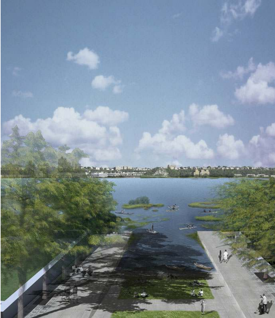
Fig. 31.6 “Marine Streets” reconfigure the ends of urban streets that are adjacent to saltwater into slowing, sloping infrastructure elements. These include coastal habitats of salt tolerant plants. The street ends are public park amenities that are resilient to the expected increasing changes in ocean levels near our cities (Reproduced from Wilks 2011. Published with kind permission of © Ecological Restoration 2011. All Rights Reserved)
