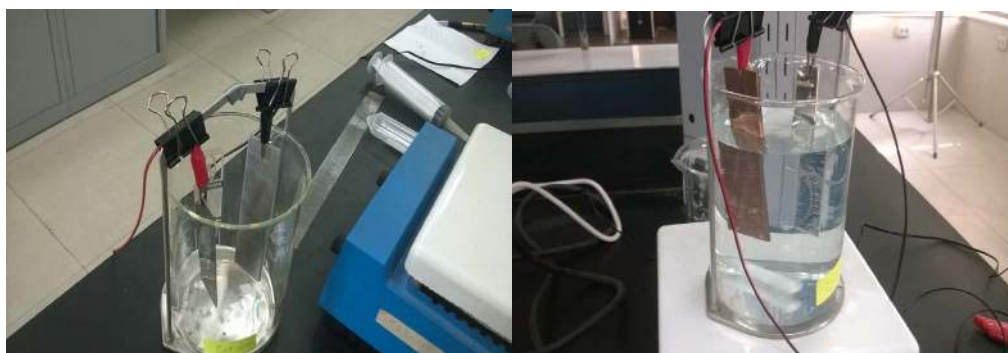
Fig. 1. Setup of electrocoagulation unit.
