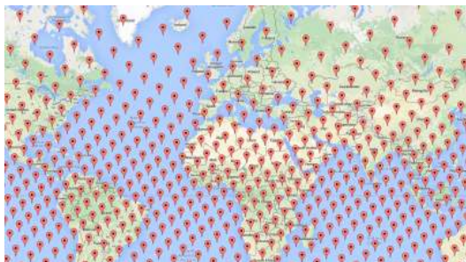
Figure 1: Example of a Fibonacci lattice overlaid on the Earth’s surface, representing the “fixed points” of a geo vector (§3.3). (Map data: Google.)
