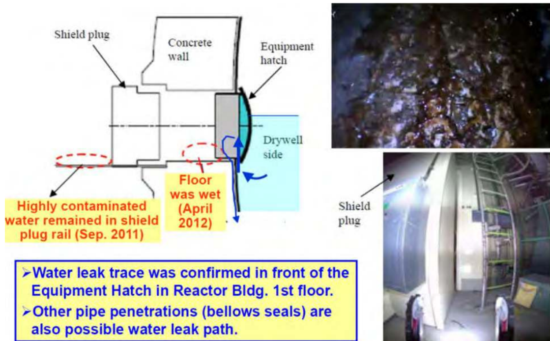
Figure 18. Liquid-phase leakage from 1F3 equipment hatch. (Courtesy of TEPCO [117])
