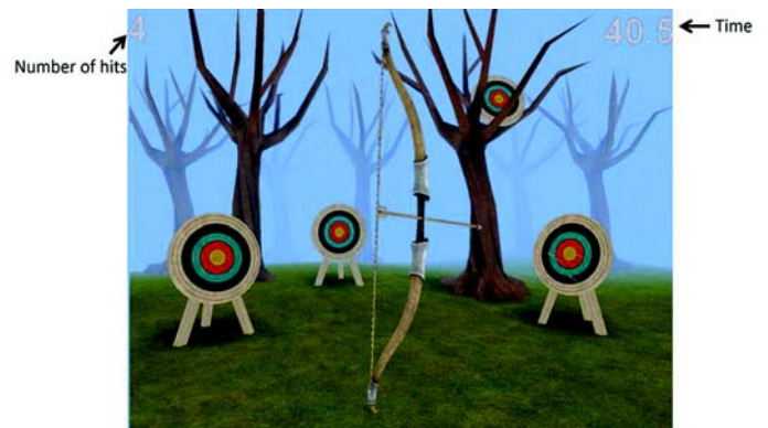
Figure 5. Archery game involved orienting bow and firing arrow by pointing hand at target and opening fingers. Game screen showed number of hits and time elapsed. Subject's arm and finger movements were detected by Kinect (Microsoft Corporation; Redmond, Washington) and P5 Glove (Essential Reality Inc; New York, New York) sensors, respectively.
