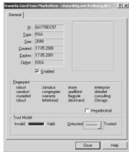
Figure 4. PGP keys: the user needs to set the trust model for the key
