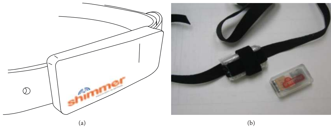
FIGURE 4: Shimmer integrated into a belt buckle (a). Shimmer attached to a Velcro stripe (b).
