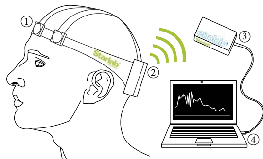
FIGURE 3: System 2—EEG analyzer. (1) Electrodes. (2) Battery pack/transmitter. (3) 802.15.4 receiver. (4) Base station.
