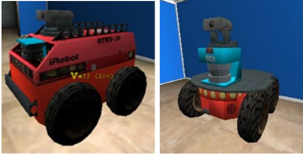
Fig. 5. On the left: a simulated ATRV Jr. On the right: a P2AT robot. Both robots mount a Sick laser in front, a PTZ camera and some sonars.
