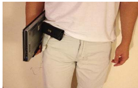
Figure 4. During data collection, a single MotionNode is packed firmly into a mobile phone pouch and attached to the subject’s front right hip
