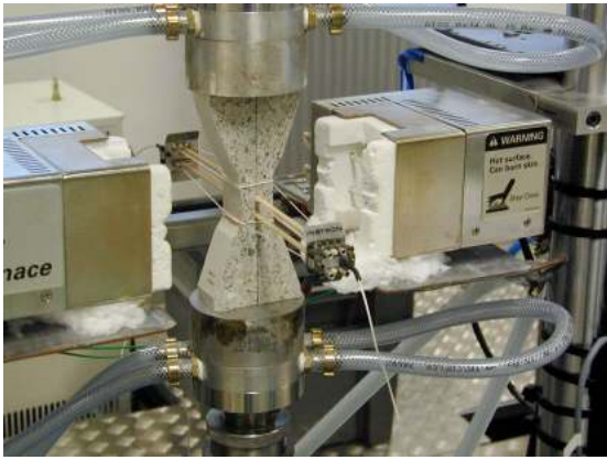
Figure 11: Zoom on the active parts of the tensile test device (left) and of the 4-point bending test device (right) in the room temperature configuration.
