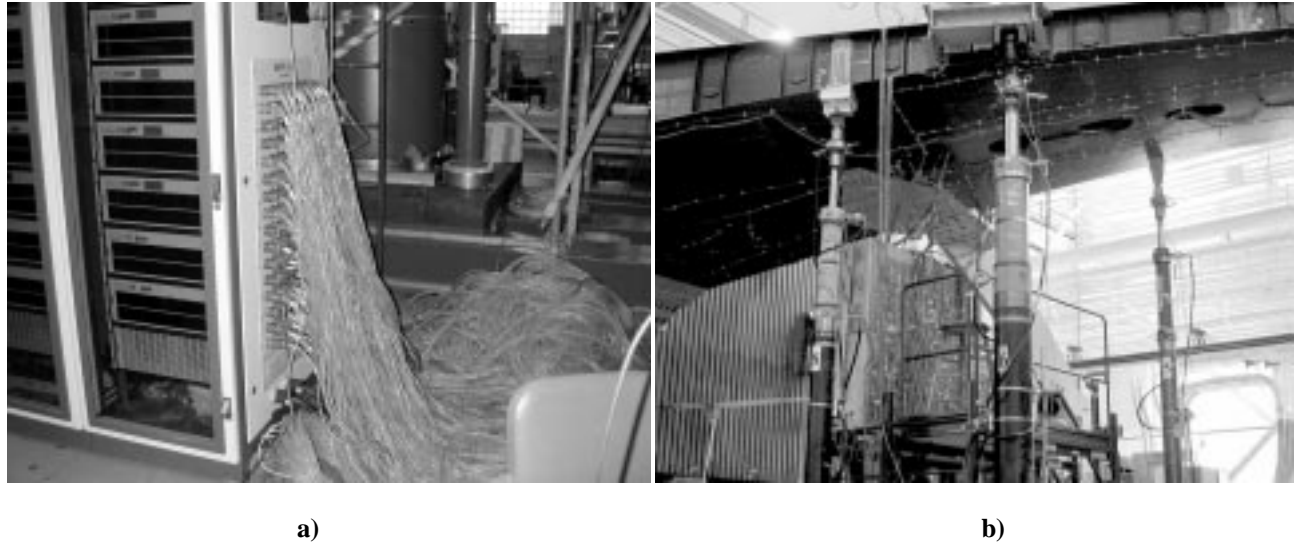
Figure 3. a) Photo showing the cabling required to connect the conventional foil gages to the ADC hardware b) Photo showing large grey connector block below the composite wing. Five oval access panel cutouts are visible running along the bottom center of the wing. The large hydraulic actuators in the foreground are two of the nine actuators used to apply the test loads.
