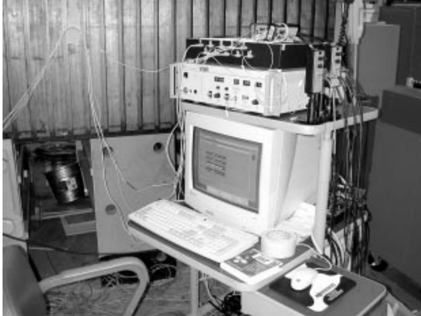
Figure 4. A photo of the optical frequency domain reflectometer on top of a computer cart in place for the test. The black box on top contained the optical network, the white rack mount unit below the optical network is the tunable laser. Seen lying on the optical network and mounted beside the laser are battery powered commercial detectors. Note the leads to the four sensing fibers taped to the wall for comparison with the bundle of wire leads required for the conventional system shown in Figure 3a.
