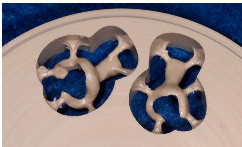
Figure 2. PEEK clasp components milled in the PEEK disk.
