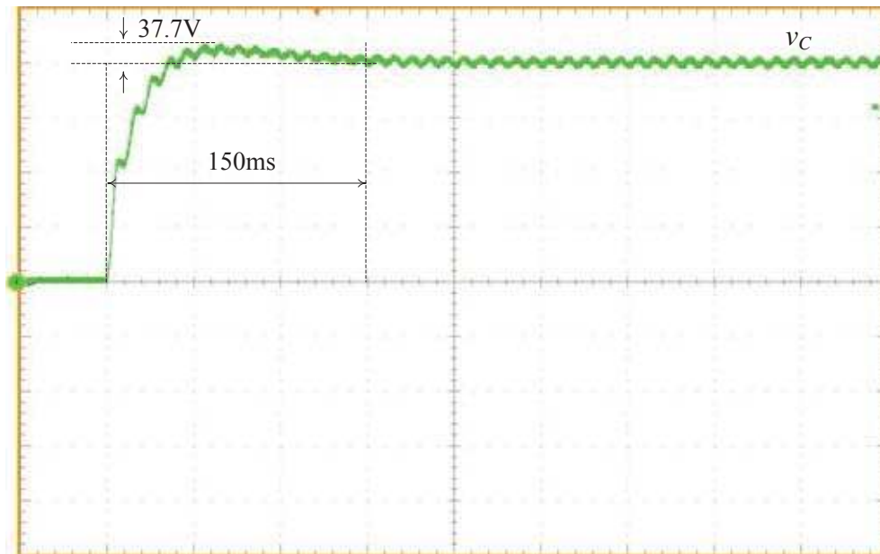
(a) Startup transient under the full load condition ( v_C : 100V/div, Timebase: 50ms/div).
