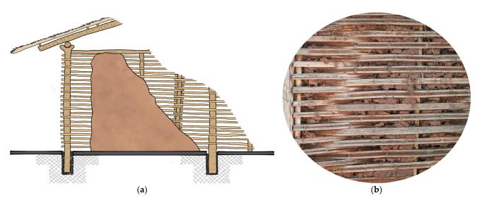
Figure 7. (a) Bajareque wall section drawing. (b) Current wall with a detached refurbishment.
