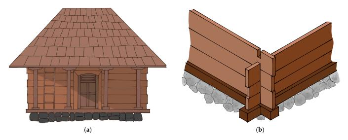
Figure 8. (a) Typical façade; (b) Technical detail of the junction between the wooden beams.
