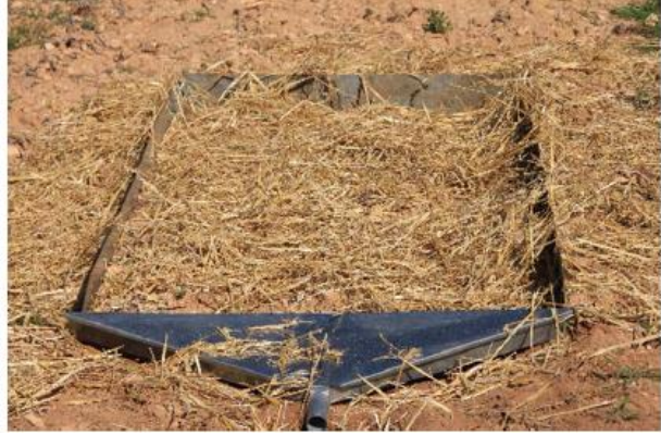
Figure 2. Plots. To the left the control (bare) plot, to the right the straw-covered plot.
