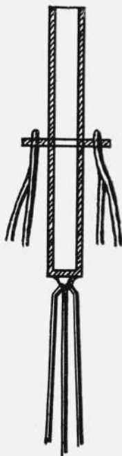
FIGURE 4. "Cleopatra-needle" assembly of Peltier junction and thermocouple for measuring the temperature of the Peltier junction.
