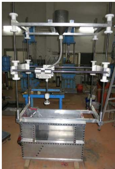
Fig. 5 Sand pluviator on the fault simulation container
