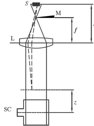
Fig. 1. Schematic diagram of the schlieren apparatus.
