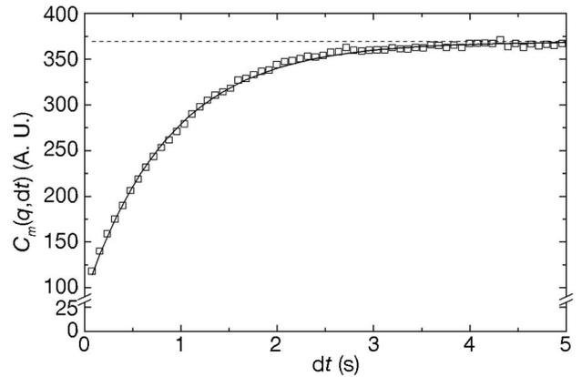
Fig. 3. Structure function  $C_m(q, dt)$  measured at  $t = 4200 \text{ s}$  as a function of time delay  $dt$ . The open squares are experimental data for  $q = 277 \text{ cm}^{-1}$ , and the solid curve is the result of fitting Eq. (10) to the data. The dashed horizontal line is the fitted limit of  $C_m(q, dt)$  for a long time delay.
