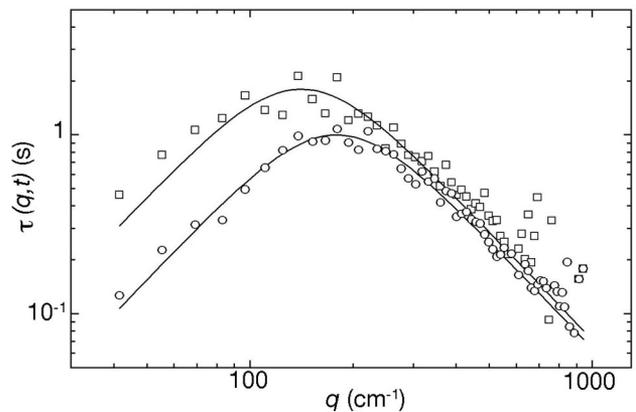
Fig. 5. Time constant  $\tau(q, t)$  as a function of wave vector  $q$  for data taken 600 s (open circles) and 4200 s (open squares) after forming the interface. The solid curves are the results of fitting Eq. (4) to the data. As time increases, the crossover wave vector corresponding to the maximum value for  $\tau$  decreases slowly, and the maximum time constant increases.
