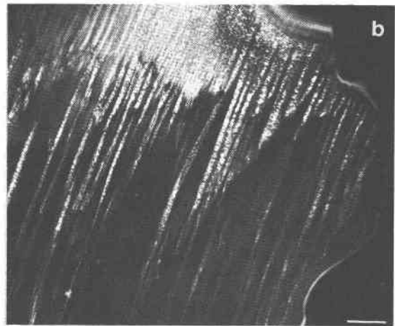
Fig. 4. Tongue and groove exsolution texture in 60°C/hr pyroxene (597-34). (a) The tweed texture is present in augite regions, and pigeonite lamellae have nucleated on defects. DF, g = 002 . (b) Same region with a P2_1/c reflection. DF, g = 102 . Scale bars are 0.5 microns long.
