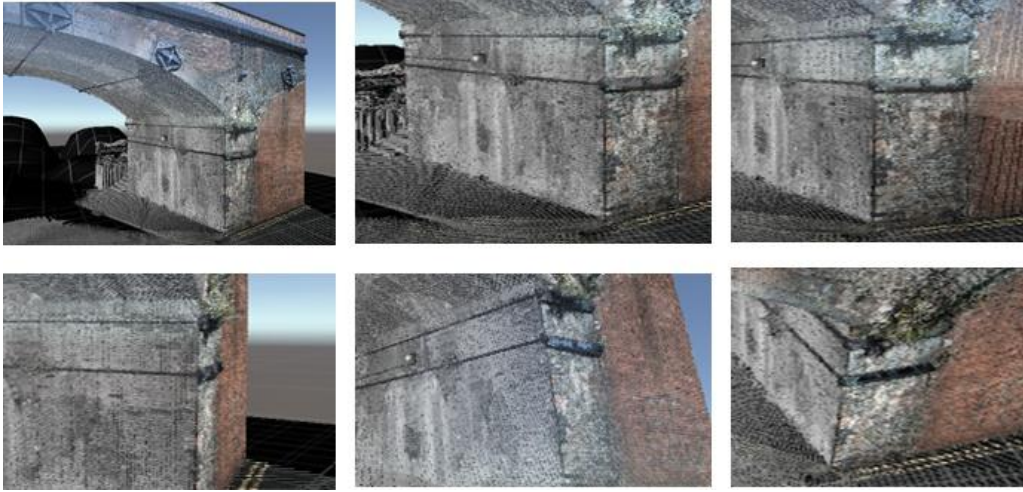
Figure 13. Interpretation of results becomes accurate as defects of interest can be viewed from multiple angles and can be discussed amongst inspectors using VR networking facility.
