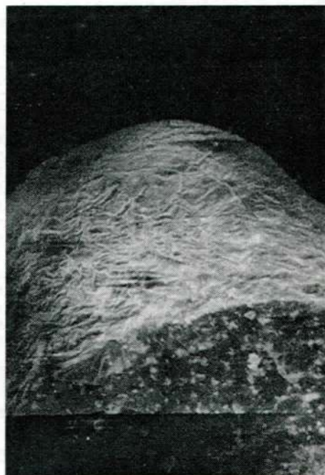
Figure 4. Surface of a ULIIIA-18 pellet (18% coating) cut through the middle and magnified 250 times.
