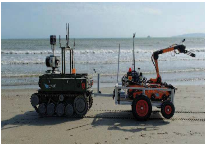
Figure 12 - ICARUS team land components: TEODOR, SUGV and trailer.
