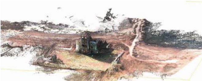
Figure 4 - Merged aerial and ground point clouds.
