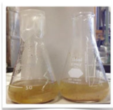
Figure 3. Flask contains 1 g tankage and 50 ml water. Each treatment was replicated three times.
