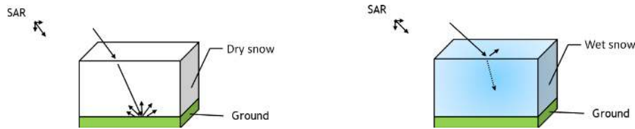
Figure 2. Main SAR backscattering mechanisms in presence of dry and wet snow at the C band. The dry snow is almost transparent, and the radar echo can penetrate the snow for several meters. The presence of LWC causes high dielectric loss, which increases the absorption coefficient.
