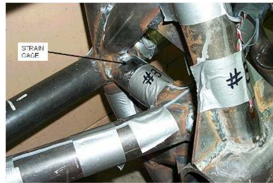
Fig. 17. Instrumentation of barrier with strain gages.
