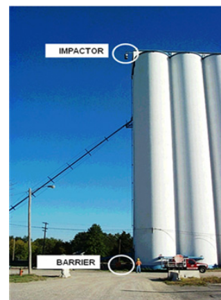
Fig. 18. The 39-meter temporary drop tower.
