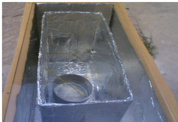
Figure 1. Inner View of the Solar Pasteurizer. The inner box and outer box are clearly visible
