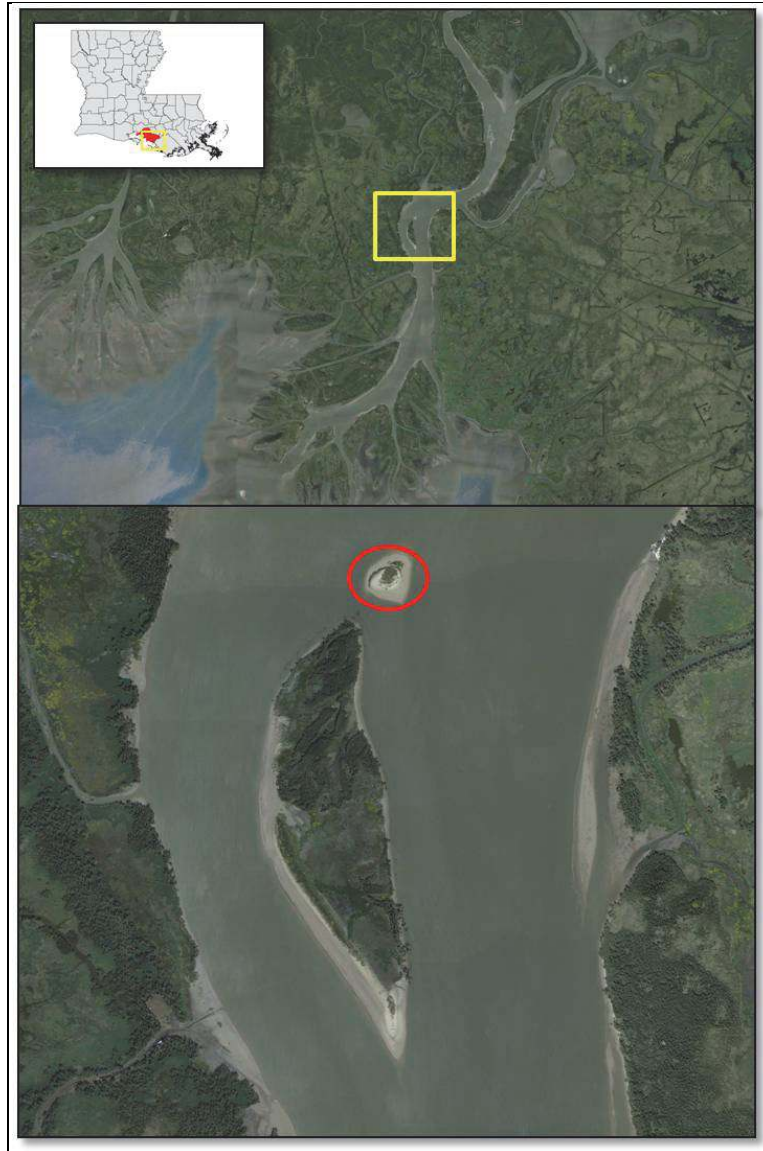
Figure 1. Study location at Horseshoe Bend Island within the Atchafalaya River, St. Mary Parish, LA (rectangle in upper photo), and a closer view of the approximately 35 ha island supported by strategic dredge material placement (lower photo). Note the small dredged material mound placed immediately upriver (north) of the island (circle).
