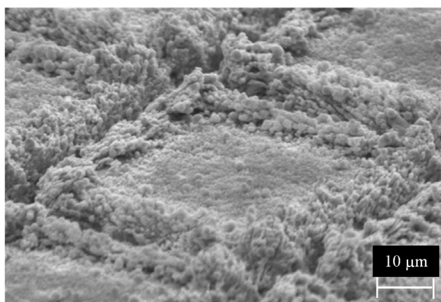
Figure 4. SEM image of brass engraved with a laser-beam spacing of 50 μm, at 12.4 W and 80 mm s -1 scanning speed, 1,900x magnification (15 kV SEM beam voltage).
