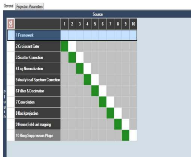
FIG. 2. Default head reconstruction chain in iTools reconstruction (Varian Inc.). Data flow from the first to the final plug-in. If plug-ins are suppressed, artifacts are created in the images.
