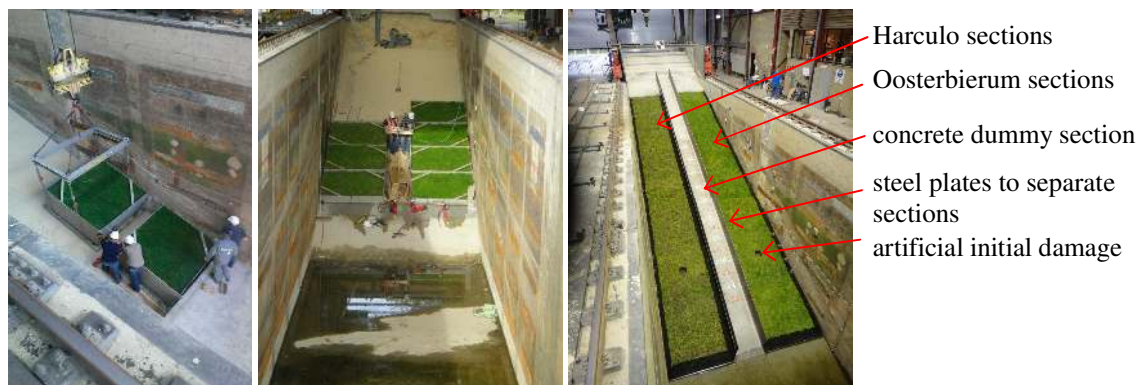
Figure 14. Placement of the grass-clay blocks in the Delta Flume.
