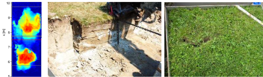
Figure 23. Left: erosion pattern at Harculo Test Section 3 in Delta Flume. Middle: sand lenses observed during collection of blocks of Oosterbierum. Right: Mouse hole
