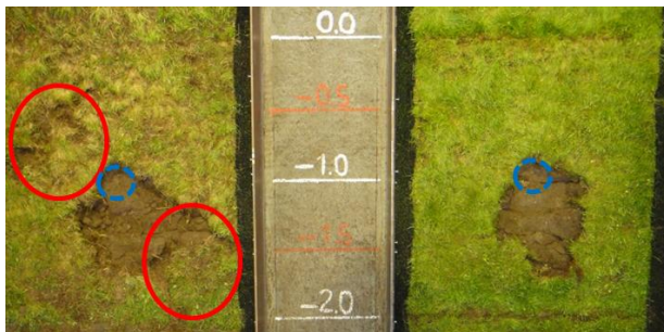
Figure 15. Damage after 1 hour at Test Section 1 (left: Harculo, right: Oosterbierum). Blue circles indicate artificial initial damage, red circle.
