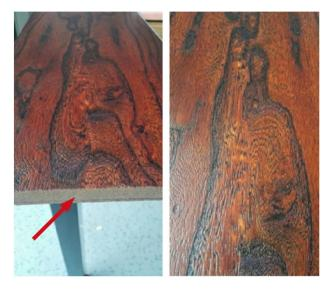
Figure 7. Elm texture 3D printed on medium-density fiberboard (MDF) substrate [66].
