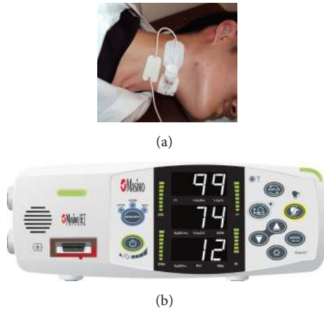
FIGURE 1: Acoustic respiratory rate monitoring device. (a) Monitoring sensor placed on the neck. (b) The display (Masimo Rad-87).
