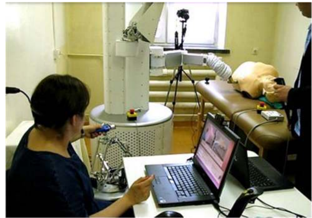
Fig. 3 Usability test with a prototype of the ReMeDi system
