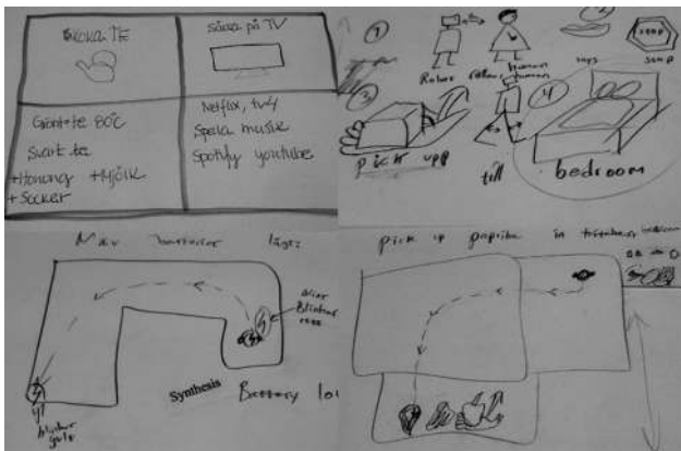
Figure 8: Four examples of sketched designs made by participants. From left to right, top to bottom: a menu system on the display with different actions, the robot could help the user with (e.g. turn on the TV), together with sub-categories (e.g. Netflix, YouTube). A pictograph system where the robot shows pictures on the display of the sub-tasks in a task that it plans to perform. A map system on the display that shows the robot's position and goal, here with the use of the label voice synthesis. A combination of a map system on the display with the robots position and goal, and pictographs at the bottom of what the robots' mission is.
