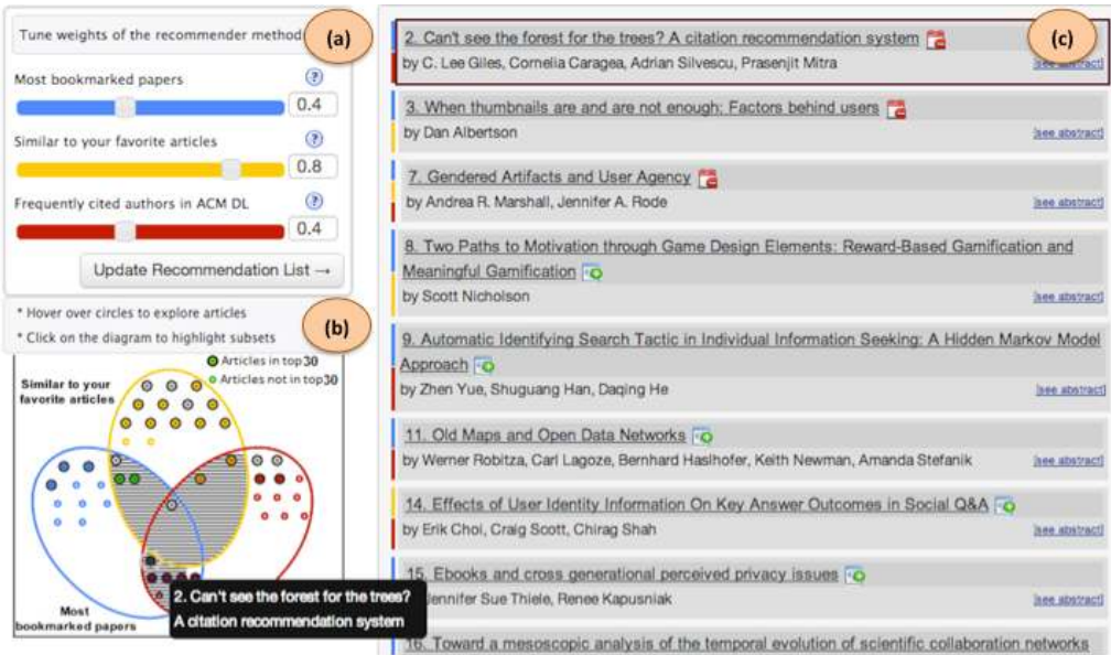
Figure 1. Screenshot of SetFusion interface. The three components indicated are: (a) sliders, (b) Venn diagram, and (c) list of recommendations.
