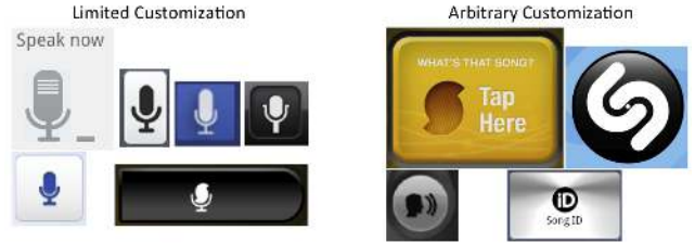
Figure 7: Customization in Android UIs. Examples of UI elements corresponding to microphone access. The ones on the left could be accommodated with a standard ACG that offers limited customization options (e.g., color). The ones on the right require significant customization, or a change to the application’s UI.
