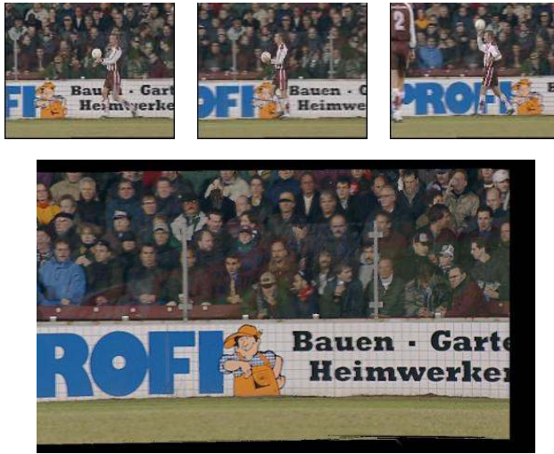
Figure 8: Broadcast: Original image sequence (top) and generated mosaic (bottom). Moving objects are removed.
