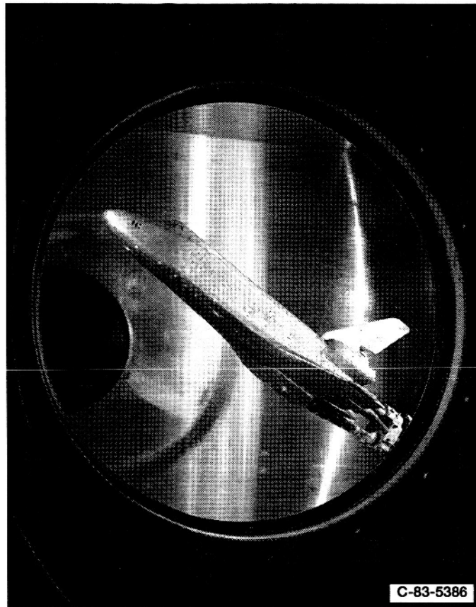
Figure 20.—Shuttle model viewed through test section schlieren window.
