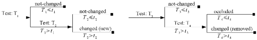
Fig. 5. General scheme for line segment based change detection. (Left) Change detection for 2D line segment in the test image. (Right) Change detection for reconstructed 3D line segments from training images. Threshold values t_1, t_2, t_3 and t_4 are selected to produce the desired change detection rate.
