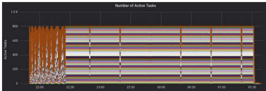
Figure 4. Number of concurrent active tasks throughout the job execution for 1 PB of input, obtained with a "readAhead" buffer of 64 KB, 804 logical cores, and 8 logical cores per Spark executor.
