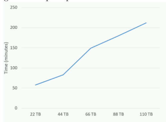
Figure 1. Performances for different input size, obtained with a "readAhead" buffer of 32 MB, 804 logical cores, and 2 logical cores per Spark executor.
