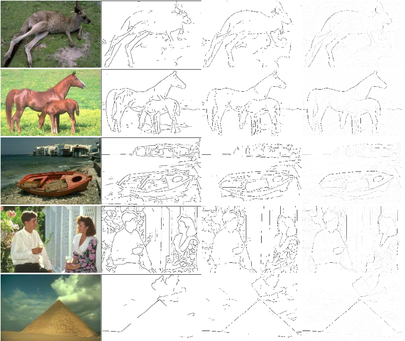
Figure 3. When compared with the local detector P_b , our detector gP_b reduces clutter and completes contours. From left to right: Original image, thresholded P_b , thresholded gP_b , and gP_b . The thresholds shown correspond to the points of maximal F-measure on the curves in Figure 2.
