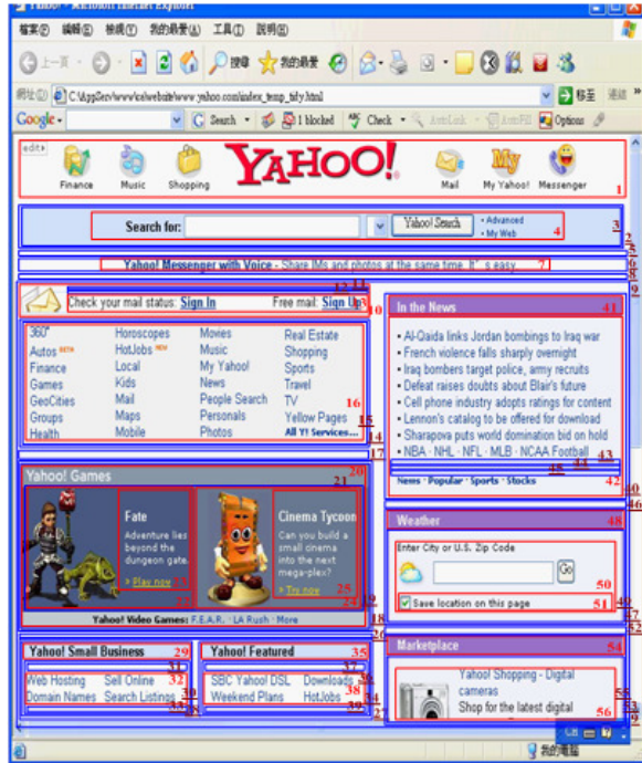
Figure 5. Example of a decomposed Web page and its corresponding object tree.
